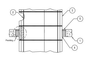
XL Insulation continuous through rated wall assembly
