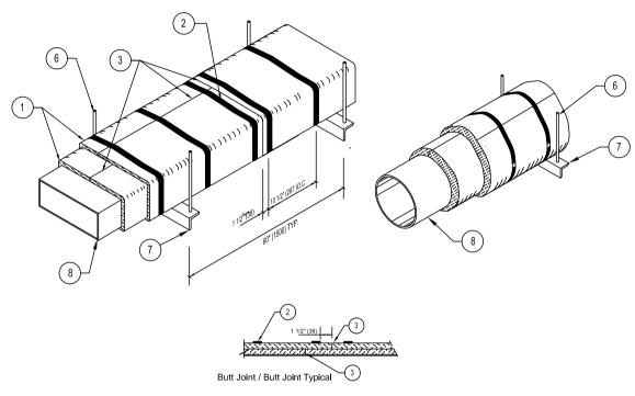
TWO LAYER INSTALLATION (Grease Duct per ASTM E2336)
